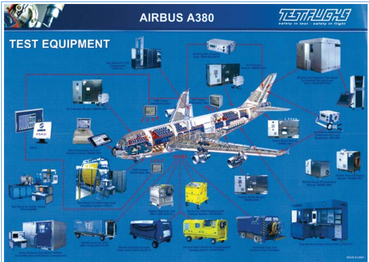
Fig. 1. Ground diagnostic and provision equipment for A-380 (drawing from the original A-380 Manual)
