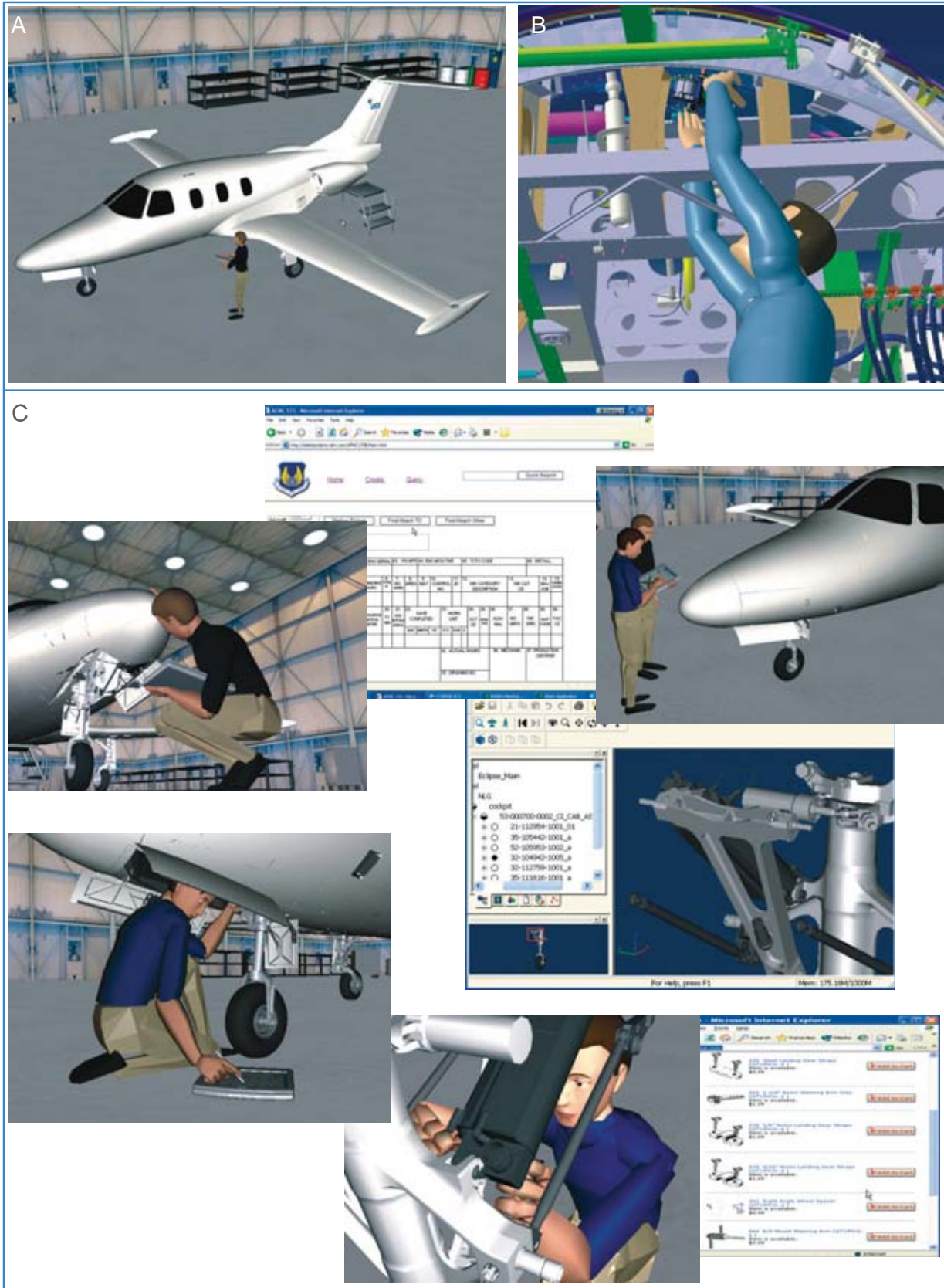
Fig. 2. Computer aided verification of an inspection of a front undercarriage (B) of an aircraft (A) and service of the B-787 aircraft (C). [By permission of UGS the PLM Company]
